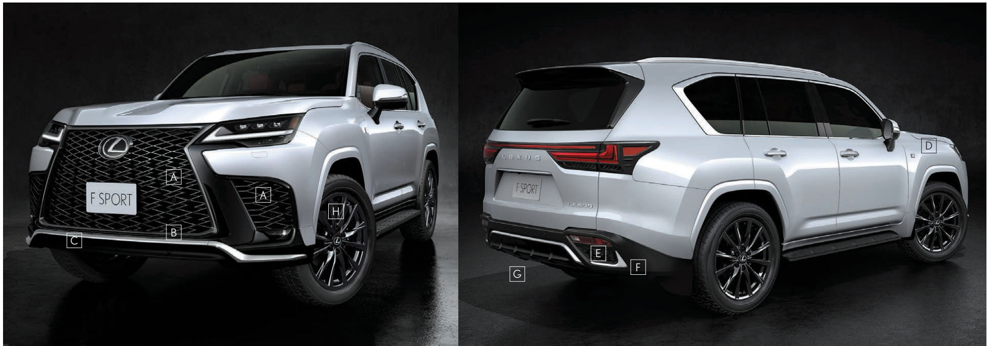
A_F SPORT-exclusive mesh grille / B_Jet black plated grille frame / C_Satin-plated molding / D_F SPORT emblem / E_F SPORT-exclusive grille pattern / F_Satin plating / G_Center cover (black material color) / H_F SPORT-exclusive 22-inch aluminum wheels
